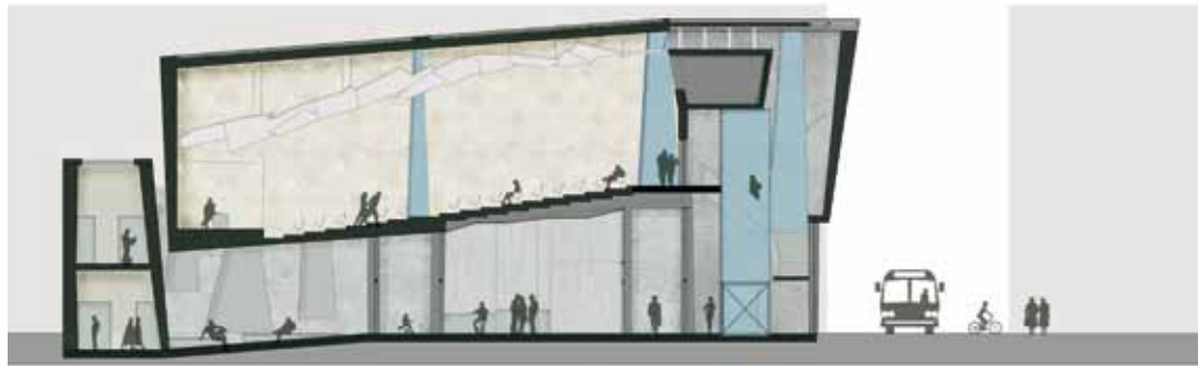
longitudinal section of the whole building. the slope in both levels leads to the focus of the Cultural Centre: the courtyard and the stage of the auditorium
